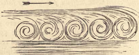
Fig. 197.—Diagram—Influence of Lateral Diffusional Aerial Whirls in Producing Aqueous Waves.
